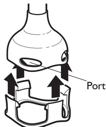
**NOTE:** Ensure Pan Guard is installed with the mounting clips positioned between the ports on the Bell Blades.
