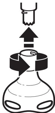
2. Insert Blending Arm into Motor Body and twist to lock until it clicks.
