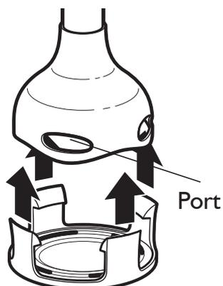
**NOTE:** Ensure Bell Guard is installed with the mounting clips positioned between the ports on the Bell Blades.
