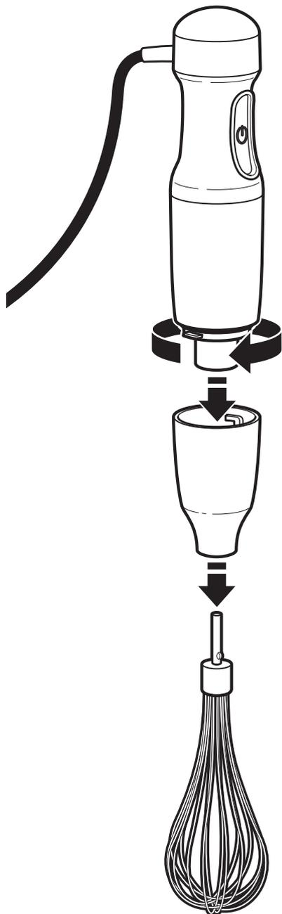
1. Insert the Whisk into the Whisk Adapter.
